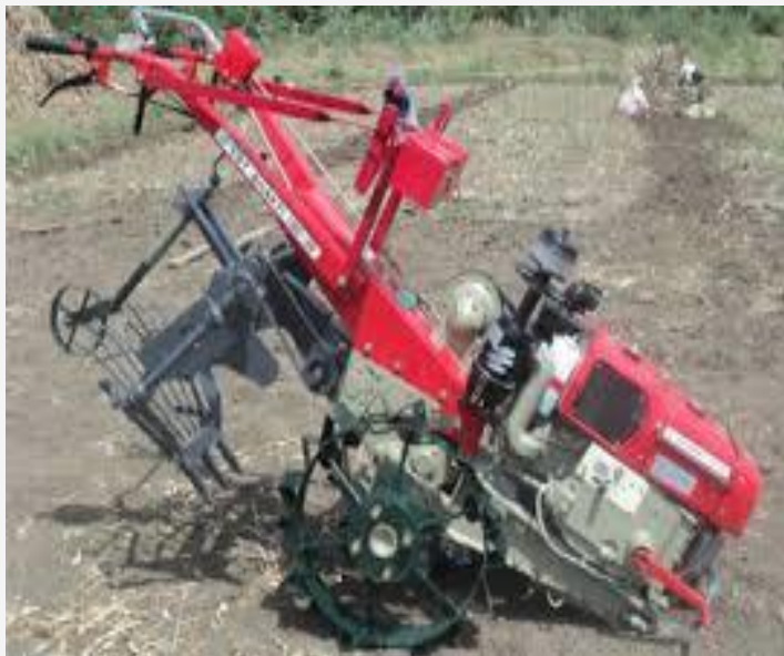
Turmeric Harvester, with belt and pulley for PTO drive
